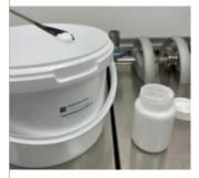
Perform preservation efficacy tests on the 2 bottles for the 2 couples bacterial strain / cosmetic product following the ISO 11930 standard or any equivalent internal method.
